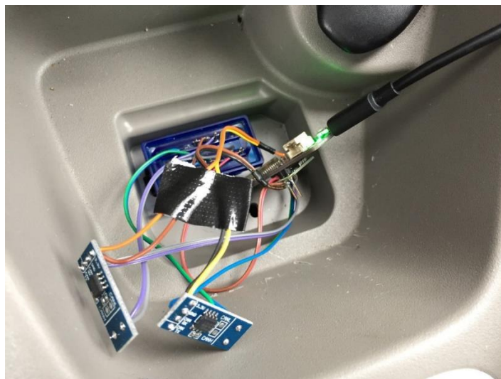
Figure 20: Data Interface without Housing plugged into the ZOE
