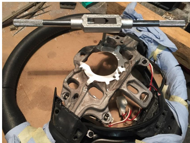
Figure 12: Steering Wheel Threading
