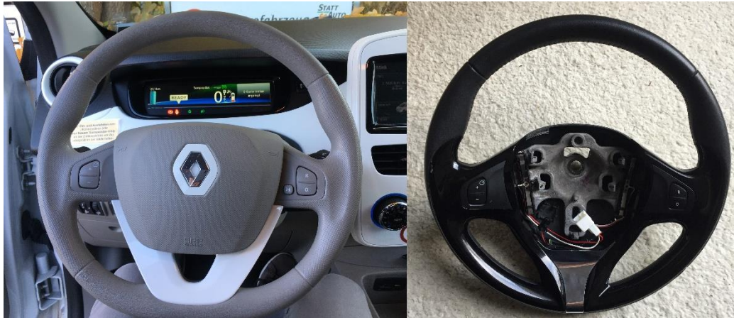
Figure 10: Steering Wheel Comparison (ZOE left, Clio IV right)
