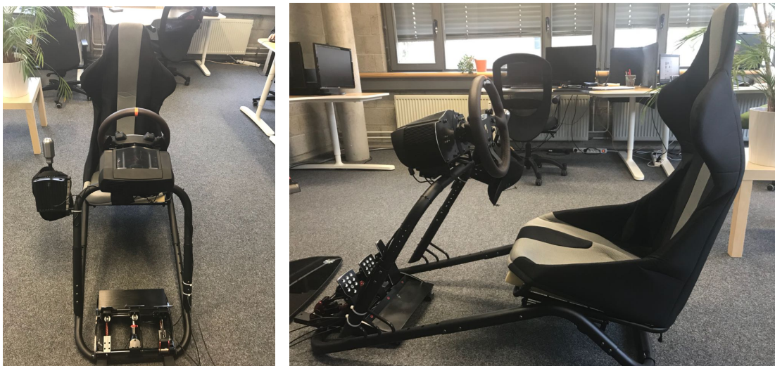
Figure 3.4.: CSL driving seat with manual speed transmission
