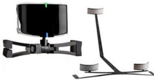
Figure 4.6.: The TrackIR head tracker: infrared camera and TrackClip
