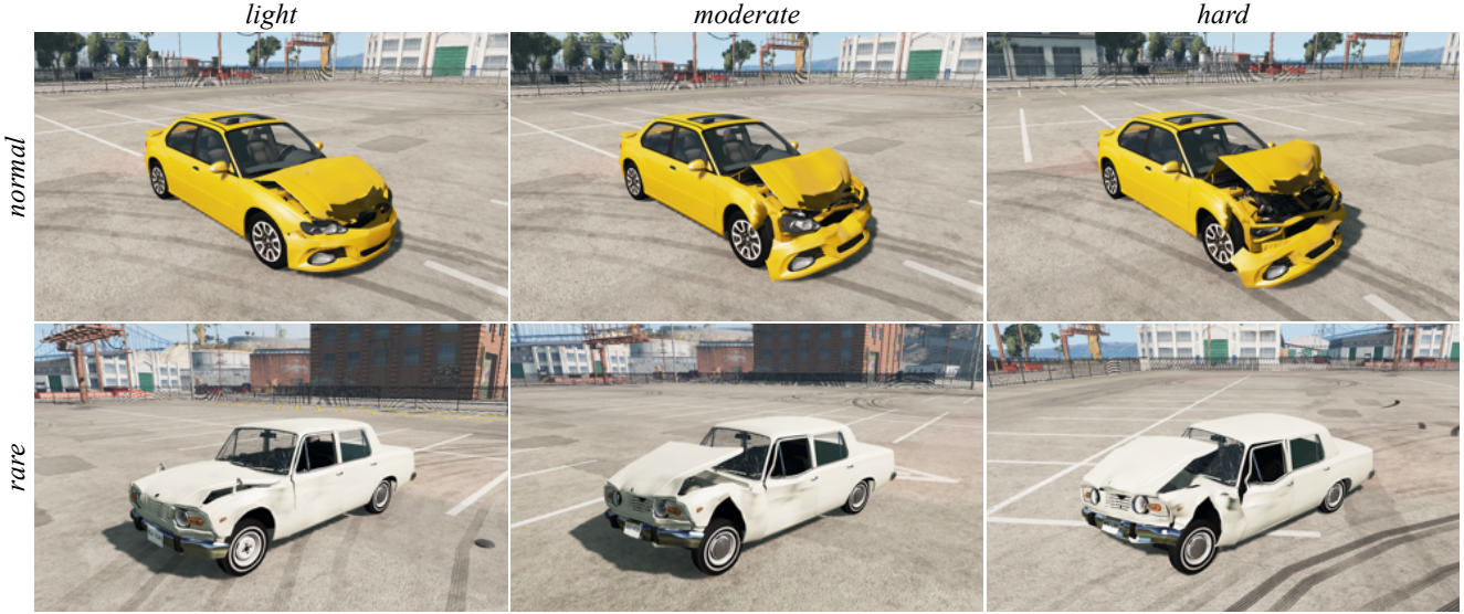
Figure 8. Comparison of linear damage intensities for normal and rare cars of CrashD. For each type of car, the accidents were created by the same hitting vehicle, coming from the same angle. It can be seen that the hard crash compromised the structure of the weaker rare car, while the normal car absorbed the impact differently, leaving the cabin unchanged. Images used with courtesy of BeamNG GmbH.
